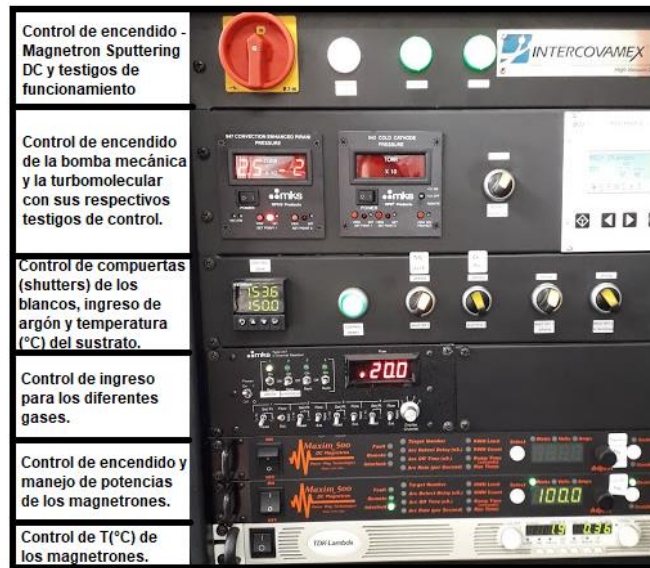
Figura 3-3: Panel de control del “DC Magnetron Sputtering”.
