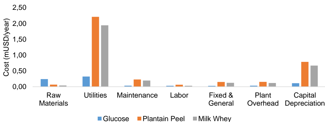
Figure 4-35. Distribution of costs in the butanol production process from each raw material at a scale of 4 ton/h
