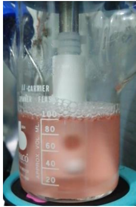
Figure 2-16: Bubble layer in Spinner flask Bioreactor with 100ml Dynamis® culture medium at 37°C, 100rpm, and 0.44ml s -1 .
