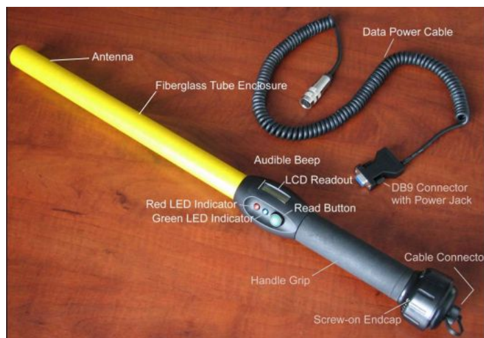
Figura 5-3: Lector Allflex RS320 RFID 11784/5
