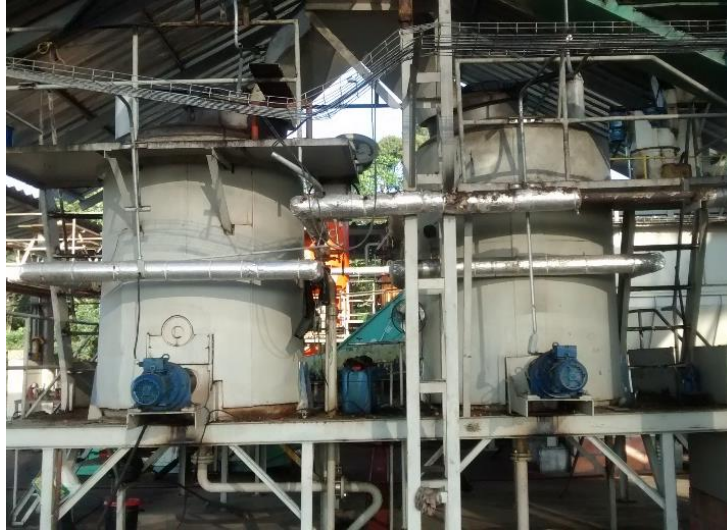
Figure 2-6. Sterilization equipment used to cook the fresh fruit bunches.
